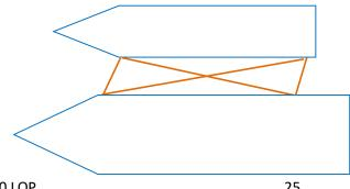
Prior to rafting a vessel alongside the rescue vessel, the skipper will conduct a crew resource meeting to discuss the size of the vessel to be rafted, the number and position of lines and position of fenders.
