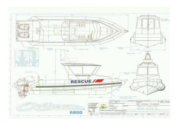
Length Overall (LOA): 6.8 meters Rear work deck length: 2.00 meters
