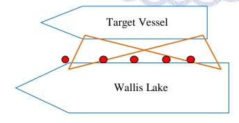
Prior to rafting a vessel alongside the rescue vessel, the skipper will conduct a crew resource meeting to discuss the size of the vessel to be rafted, the number and position of lines and position of fenders.
